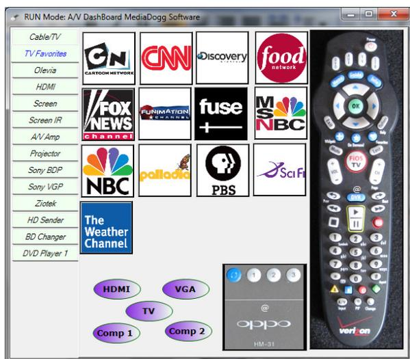
A standalone component, **a/v Dashboard** provides an Automation Editor and Virtual Remotes Editor, which presents the virtual remotes in a tabbed view. Buttons can be assigned and positioned, and infrared sequences can be captured (learned) and associated with the buttons on the virtual remote tabs. This component also supplies Remote Automation Services to other **a/v Automation System** components.
